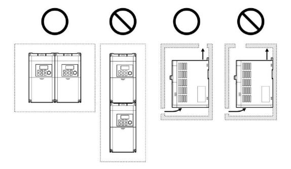
• If you are installing multiple inverters in one location, arrange them side by side and remove their top covers (optional). The top covers MUST be removed for side-by-side installations. Use a flat head screwdriver to remove the top covers.
