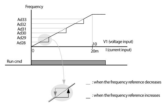
Use frequency jump to prevent motor operation at mechanical resonance frequencies. When jumping through a frequency bands while a motor accelerates and decelerates, operation frequencies cannot be set within the preset frequency jump band and the inverter operates at a constant speed.
