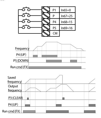
When the Ad66 code is set to 1: The motor accelerates by as much as the step frequency set by the Ad67 code at the multi-function input's positive edge that has been set as the Up terminal signal. The motor decelerates by as much as the step frequency set at the Ad67 code at the multi-
