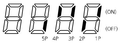
※ Only 1P–3P are available for models equipped with standard I/O.
