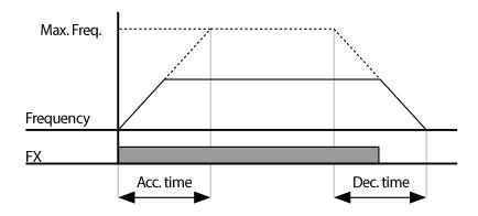
It is particularly useful that the time scale unit changes based on the max 5 digits of Acc/Dec time value when more accurate Acc/Dec times are required due to load characteristics.
