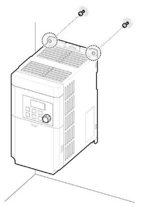
Mount the inverter on the wall or inside a panel using the two upper bolts, and then fully tighten the mounting bolts. Ensure that the inverter is placed flat on the mounting surface, and that the installation surface can securely support the weight of the inverter.
